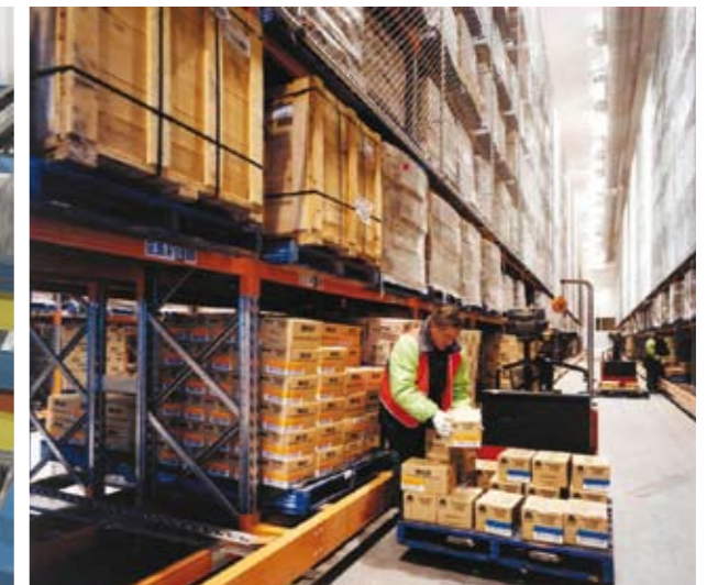
Pallet Live Storage First in, first out automatic stock rotation
